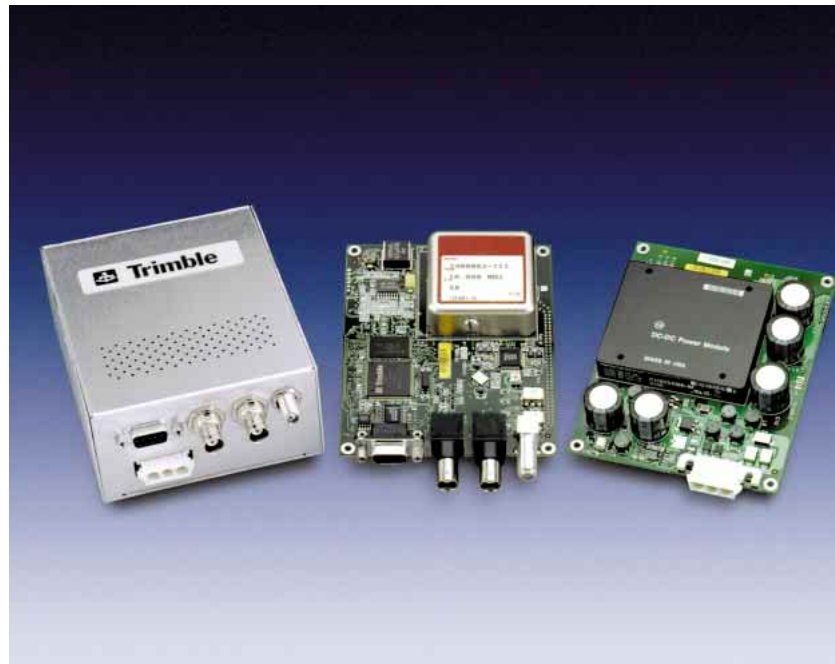
Trimble's Thunderbolt™ GPS Disciplined Clock in enclosure, in board form, and 24V power supply.
